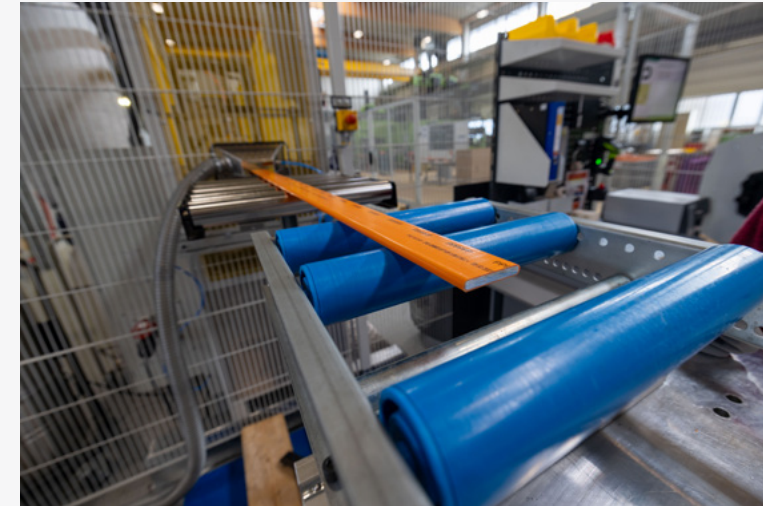
Finishing of the sheathing of aluminum rails at the Braunau plant, Austria.
