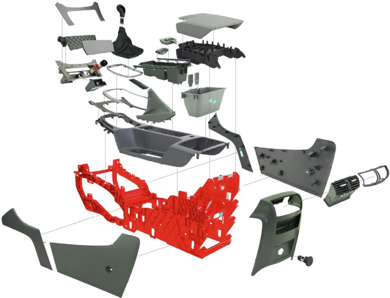
FIGURE 2 Exploded view of a centre console with conventional support element design (structural component shown in red)
