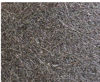
4 Macro shot of the fine kenaf fibre structure with laminated decorative film
