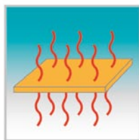
2. Pre-pressing and heating to a NF-PP mat
