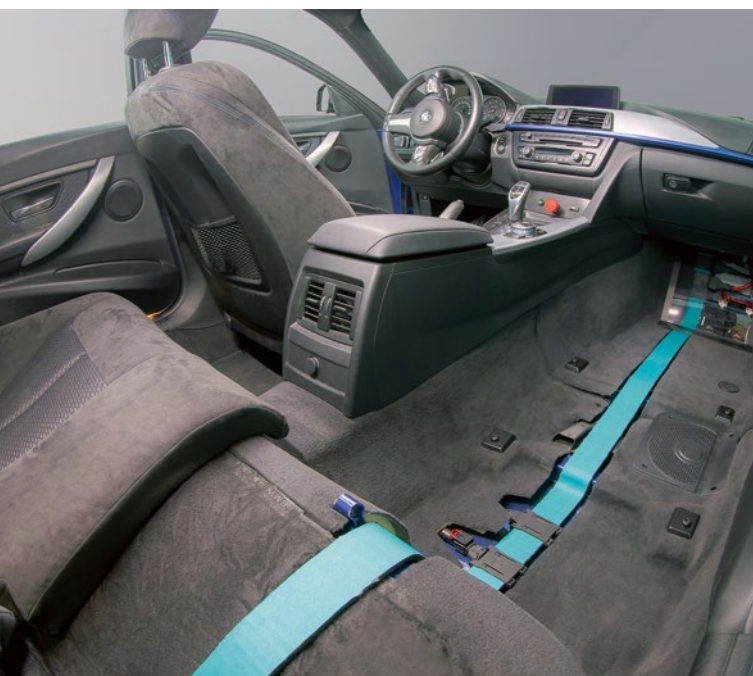
FIGURE 5 Use of bus-bars and electronic power distribution in Dräxlmaier Smart KSK (© Dräxlmaier)
