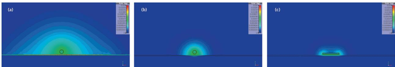
FIGURE 4 Field spread with round single conductors via one steel and aluminium sheet, as well as a single flat conductor via aluminium sheet at 1 kHz (l. to r.) (© Dräxlmaier)
