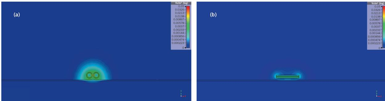
FIGURE 5 Field spread at 1 kHz with a double round conductor and a double rail on a sheet of aluminium (© Dräxlmaier)
