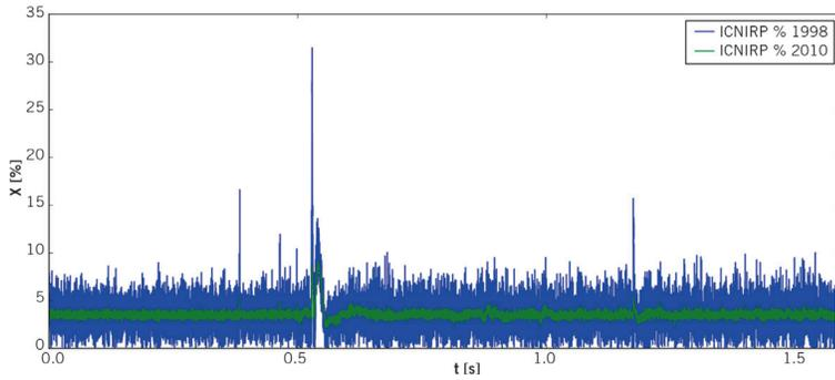
FIGURE 7 Comparison of measured values according to ICNIRP 1998 and 2010 (© Dräxlmaier)
