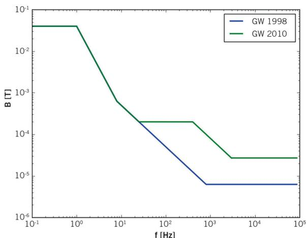
FIGURE 6 ICNIRP limits for magnetic flux density  $B$  in Tesla as a function of frequency for both versions of the directive (1998/2010) (© Dräxlmaier)
