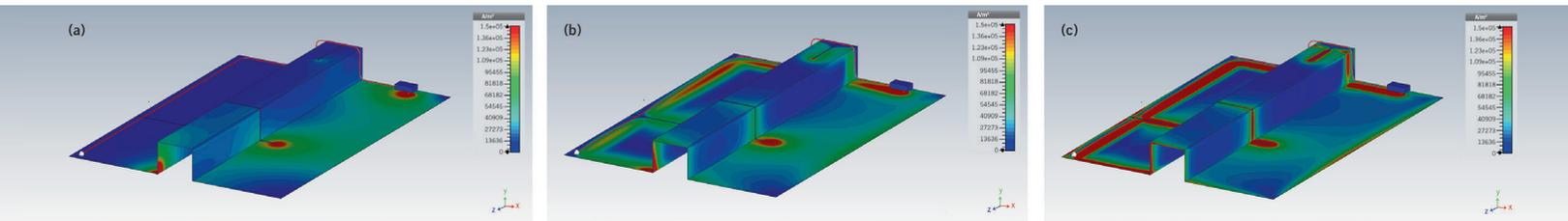
FIGURE 3 Current density 5/50/200 Hz in an aluminium plate with imperfections (© Dräxlmaier)
