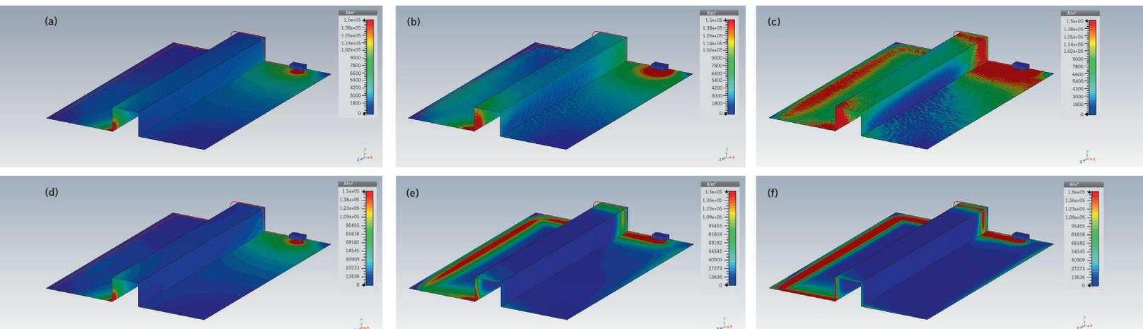
**FIGURE 2** Current density 50/200 Hz (top steel/bottom aluminium) (© Dräxlmaier)
