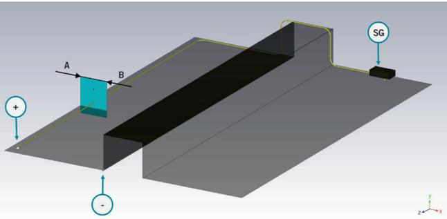
**FIGURE 1** Schematic diagram of simulation set-up: (+) B+, (-) earth, (CU) control unit, section AB (level for further considerations) (© Dräxlmaier)
